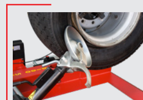
Manual tool arm movement with quick unlocking system
