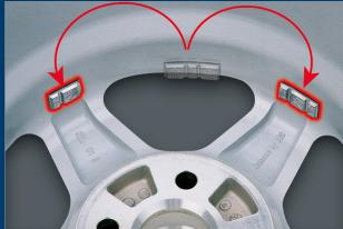
**ALU-S and SPLIT programs:** thanks to an intelligent gauge, the machine automatically detects if an alloy rim is used and calculates distance and diameter for both correction planes. The SPLIT function re-calculates the unbalance on the basis of selected number of spokes, in order to correct behind the two nearest spokes
