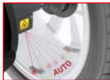
Laser spotter to indicate the exact position for stick-on weights application inside the rim
