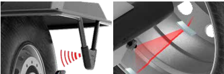
LA sonar device for automatic wheel width measurement and, with laser pointer, for measuring the lateral eccentricity of the tyre shoulder
