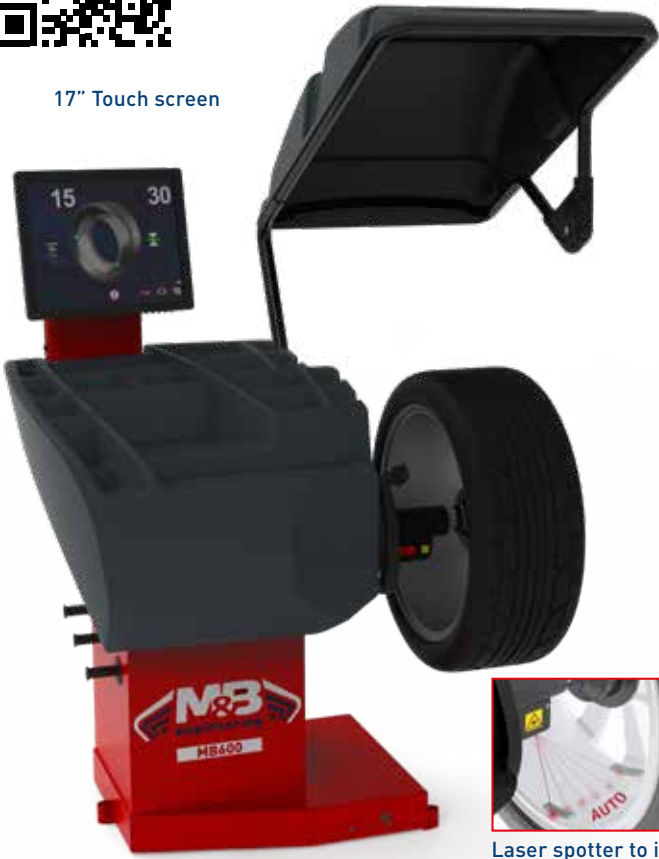
Laser spotter to indicate the exact position for stick-on weights application inside the rim
