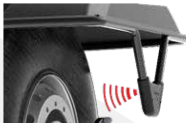
LA sonar device for automatic wheel width measurement and, with laser pointer, for measuring the lateral eccentricity of the tyre shoulder
